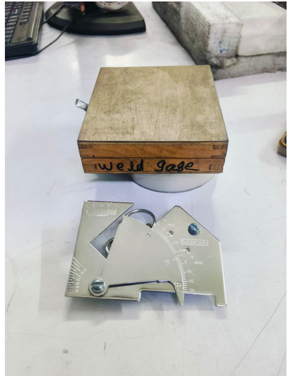
Photo 2: Welding Gauge Set (Fillet / Butt Weld Gauge, 0–20 mm) Used for measurement of fillet weld size, reinforcement and root gap during weld inspection
