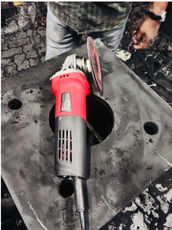
Photo 3: Angle Grinder in Use on Bearing Base Plate Edge preparation, deburring and surface finishing of machined / gas-cut steel plates
